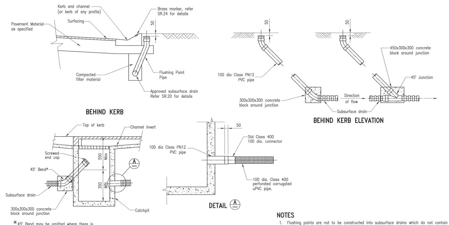
\*45\* Bend may be omitted where there is insufficient depth to the subsurface drain trench. A minimum fall of 100mm is to be provided in the connection pipe between the cap and the subsurface drain pipe.
