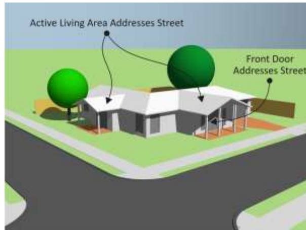
Figure 12.3.5.1.5— Orientation of Habitable Rooms and Balconies and Verandahs to the Street
